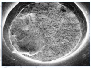
A typical hydrogen embrittlement fastener fracture.
